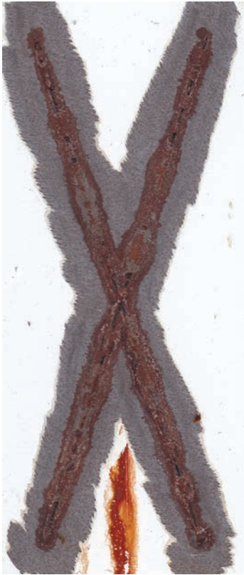
Commercial Primer (containing 10% \text{ZnPO}_4 ) + Top coat
